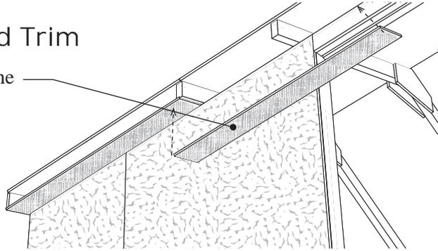
2. Install (1) one 1x4x47-1/4" and (1) one 1x4x72" long gable trim, flush with the top of the roof sheathing on each end wall. Use 8d galv. nails.
