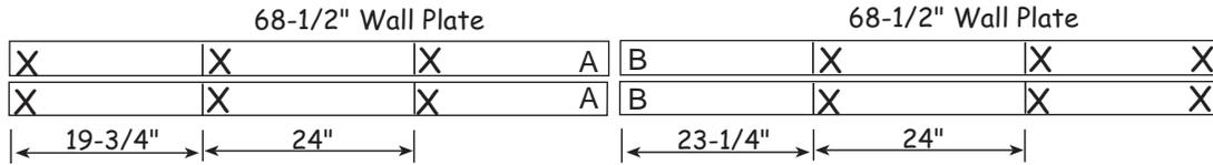
2. Install 52-7/8" long wall studs, between the wall plates, over the 'A', 'B' and 'X' marks. Use 10d sinkers. Nail wall frames together.
