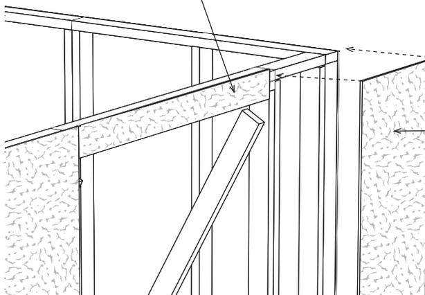
7. Install a full width x 4-3/4" siding panel over the door header. Install 1" above top of 2x4.
